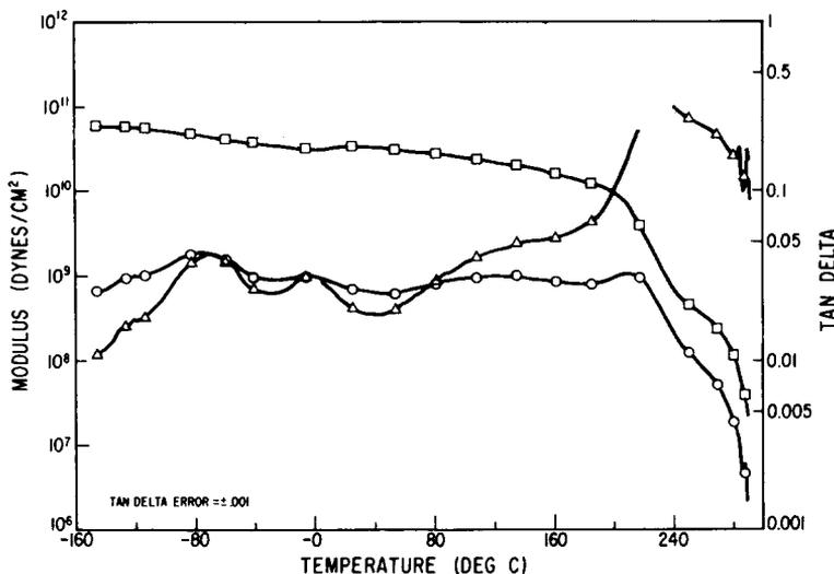
Fig. 3. Plots of Young's storage modulus, loss modulus, and  $\tan \Delta$  vs. temperature for Methocel HG with 25%  $\beta$ -cyclodextrin film.  $\square$ , Storage modulus;  $\circ$ , loss modulus;  $\Delta$ ,  $\tan \Delta$ .  $\tan \Delta$  error  $\pm 0.001$ .
