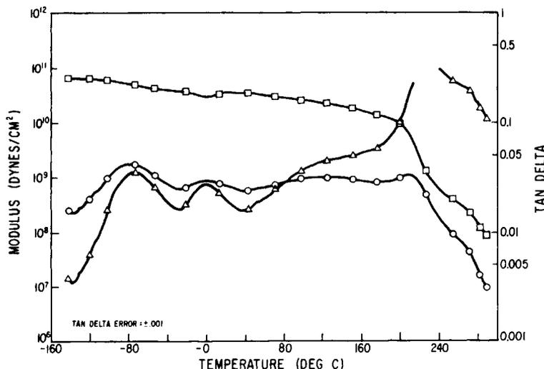
Fig. 2. Plots of Young's storage modulus, loss modulus, and  $\tan \Delta$  vs. temperature for Methocel HG with 25%  $\alpha$ -cyclodextrin film.  $\square$ , Storage modulus;  $\circ$ , loss modulus;  $\Delta$ ,  $\tan \Delta$ .  $\tan \Delta$  error  $\pm 0.001$ .
