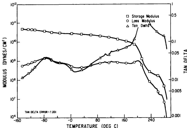
Fig. 1. Plots of Young's storage modulus, loss modulus, and  $\tan \Delta$  vs. temperature for Methocel HG film.  $\square$ , Storage modulus;  $\circ$ , loss modulus;  $\Delta$ ,  $\tan \Delta$ .  $\tan \Delta$  error  $\pm 0.001$ .
